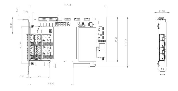
Dimensions are in millimeters.
